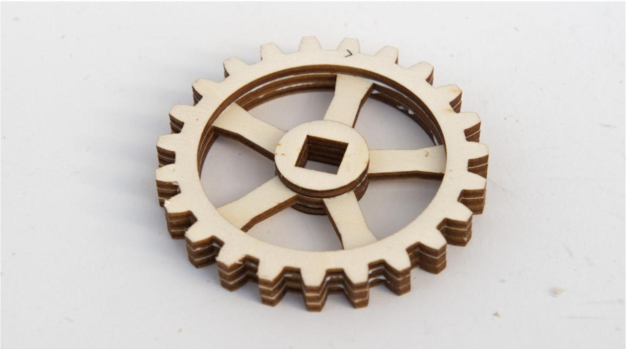
Glue together the six layers of the cam, make sure the hole is accurately lined up.
