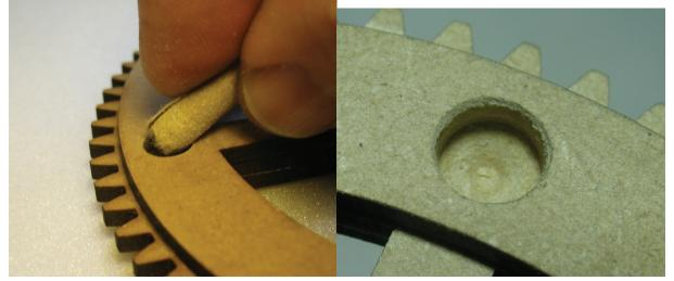
Insert the wheel between the uprights and push the axle pin through the wheel. It is a tight fit so make sure you support the rear upright whilst pushing the pin in place.
