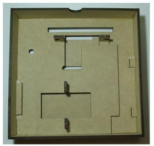
Glue the side pieces together and onto the top piece. The bottom piece should NOT be glued as it must be removable for access to motor and batteries. However it can be used to keep the base parts aligned while the glue dries. Hold the parts together with strong rubber bands.
