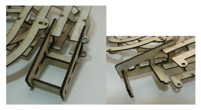
Glue the seesaw parts together as shown below. Carefully thread the M4 nut onto the prong. If it is very tight, sand the prong a little bit. The nut acts as a counterbalance and by moving it along the prong you can balance the see-saw so it tips when 3 ball are on it.
