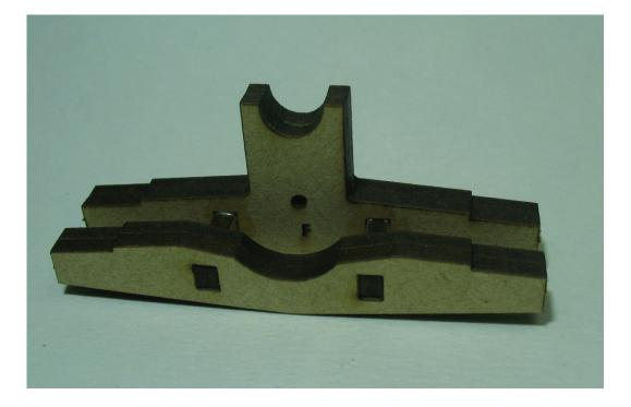
Glue the switch frame onto the upright. Sand the exit hole and frame so there is a smooth downwards slope. Only light sanding is required.
