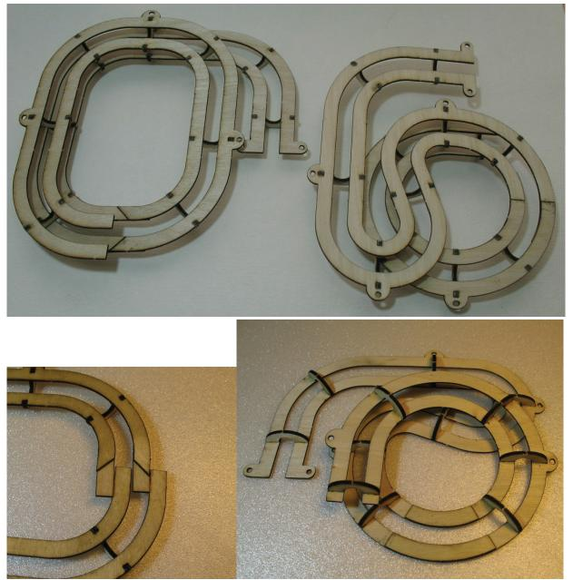
Glue the end doublers onto the zig-zag track pieces. These go on the side of the sheet marked with an X (opposite side of the spacers!).
