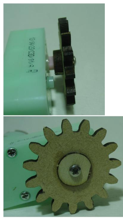
If you find that the mesh with the large gear is a little on the tight side, a spacer or two cut from thin card can be placed under the motor.
