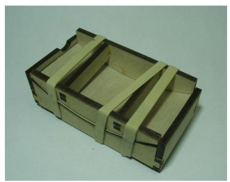
Now sand the ply so it is flush with the front and rear of the tray. Glue the front MDF piece in place. The cut-out should face left as shown in the picture
