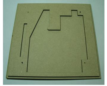
The top part of the base consists of three pieces. Glue the top and doubler together, using short pieces of carbon rod for alignment as with the bottom. Add the motor/battery retaining part. The rubber band hooks take care of the alignment. Cover the 1.5mm holes with the small MDF pieces supplied.
