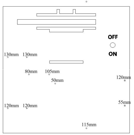
Push the rods into the holes in the base. Don't glue them in place. It is easiest to do the zig-zag track first, then remove it and do the track with the accumulator. It gives you more space to make adjustments.
