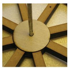
Very lightly chamfer/round the lip of the holes sp they are smooth. This is done with a scrap of sandpaper rolled around a suitable round object like a pen.
