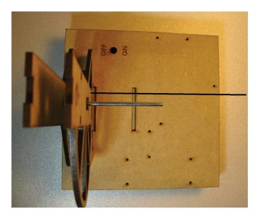
The bottom of the base can be used to ensure the front upright is square to the base. A couple of rubber bands will hold it in place. Don't glue the top piece in place yet so you avoid having to cut the rubber band.
