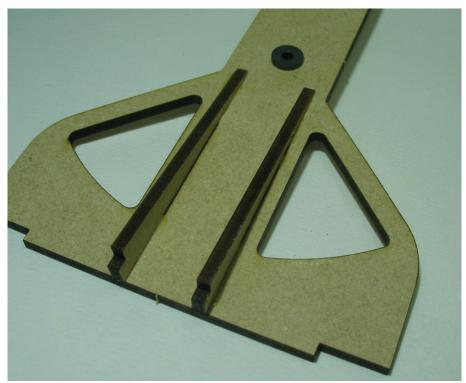
Glue the uprights onto the base. Insert the 3mm rod in the bearings. The front upright can be slid a bit left/right. Slide it so the rod spots parallel with the base sides. This ensures the wheel runs true between the uprights.
