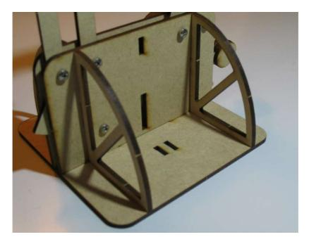
Assemble the trigger in the same way you assembled the frame. You have the option to use a trigger lever with a string pull or a push button trigger lever. Glue the trigger lever supports onto the base.
