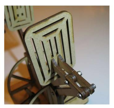
Do up all the nuts until the parts still move freely but with minimal sideways wobble. Better a bit too loose than too tight as MDF can expand in humid conditions and make the motion stiff.
