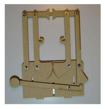
Place the remaining side frame and horisontal arms onto the bolts and screw on the nuts. Do not tighten them at this point.
