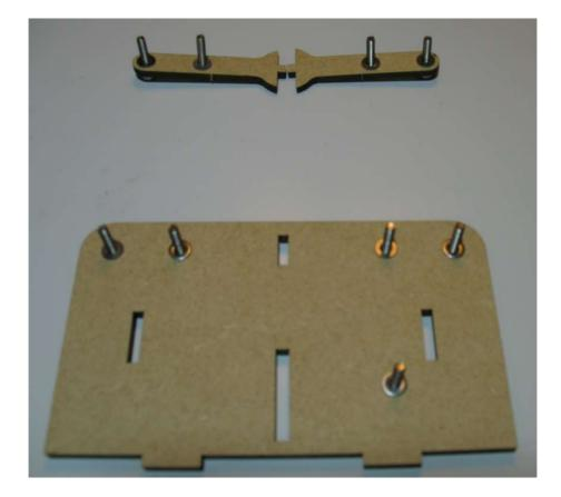
Place the vertical arms and trigger arm onto the bolts. Ensure the toothed arms mesh as shown on the picture. Add a washer onto each bolt.
