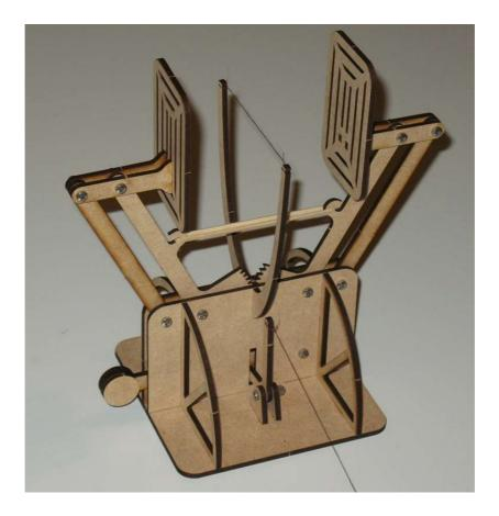
**Please note:** All the assembly can be done with PVA glue. Don't apply it from the bottle or tube but put a blob on a piece of plastic and apply it with a small brush. That way it is much easier to control the amount of glue you apply.
