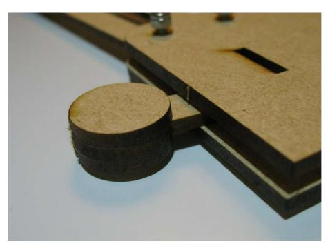
Glue the four supports onto the side frames and then glue the whole assembly onto the base. Do it in on go before the glue sets so you have time to wriggle the parts around so the tabs enter the slots. Do not put glue on the tabs themselves as this can cause them to expand and make it difficult to insert them into the slots.
