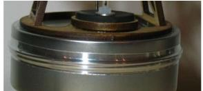
The displacer should not touch the can at each end of its travel. Insert the bent section of the displacer rod into a hole in the connecting rod so the displacer does not touch the bottom or top of the tin at the ends of travel
