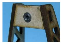
Insert the 2mm axle so it protrudes an equal amount on each side. Check that the axle spins freely. If it doesn't there may be a bit of misalignment between the bearings. Wriggling the axle from side to side and up and down to align them.
