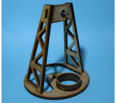
MDF is not moisture resistant so now is a good time to paint the engine parts. If you prefer the plain MDF look you can use a clear lacquer or MDF sealer. For colour, acrylic automotive paint in a "rattle can" works well. If you use spray paint, roll up a piece of paper and insert it into the hole for the bearings so you don't get paint into the bore.
