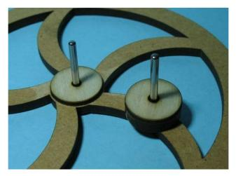
Fit the 2mm crank pins into the flywheel and crank disc. If using pliers to push them in, the pliers should have smooth jaws so they don't damage the pins. Alternatively you can tap them in with a small hammer. Put a scrap piece of MDF between the pin and the hammer so you don't damage the pin. Take care to ensure they go in at right angles to the crank disc and flywheel and that you don't break the thin wall between the holes.
