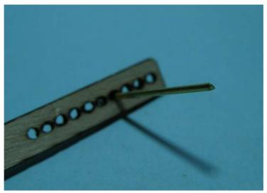
Glue the parts together using a ball bearing and the brass wire to keep parts aligned. Use glue sparingly so it does not fill up the small holes and/or gets into the ball bearing.
