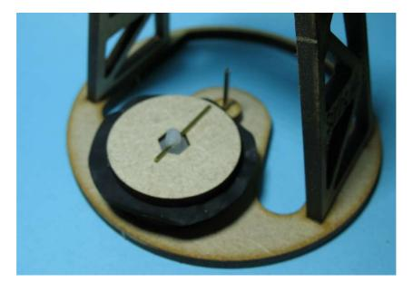
Slide the disc around until it aligns with the rings. You can now fit the diaphragm retainer rings. Once they are in place, slide out the brass wire and remove the alignment disc.
