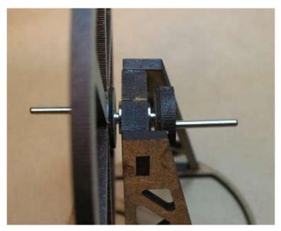
You can use an off-cut from the 0.8mm plywood sheet that holds the connecting rods as a spacer when you mount crank disc and flywheel. It will give you the desired gap between crank disc/flywheel and the bearings. Remember to remove the spacer afterwards
