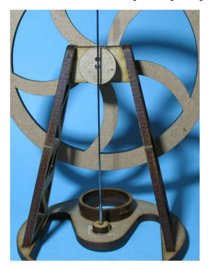
Insert the hypo in the base plate from the underside. Push it in so it sits flush with the underside. Do not add glue at this point. Use the piano wire displacer rod to ensure the hypodermic tube aligns with the centre of the axle and is square to the base plate. If it is not aligned properly the displacer will be tilted and could rub against the side of the tin. Once you are sure it is properly aligned, glue it in place with epoxy and add the doubler to reinforce the joint.
