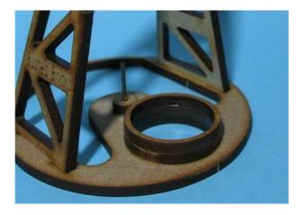
Chamfer the outside of the tabs on the uprights so they fit in the base.
